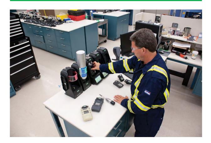
f you work with direct-reading portable gas monitors (DRPGMs) to check oxygen levels and look for toxic or combustible gases, you're likely familiar with the concepts of bump testing and calibration. But if you were given an on-the-spot pop quiz on the subject, could you tell the difference between these terms?
