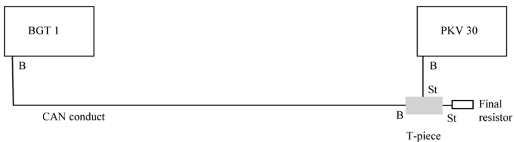
Fig. 168 Connection Suprema Gateway CAN/Modbus RTU
