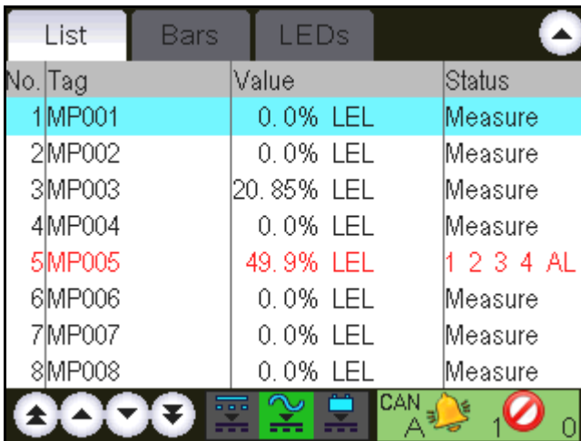
Fig. 10 List display [with a measuring point in Alarm]
