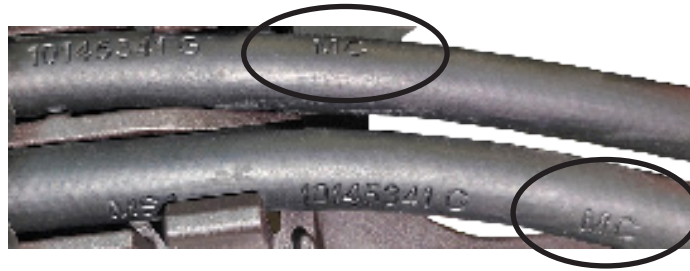
Fig. 26 High pressure line and medium pressure line marking
