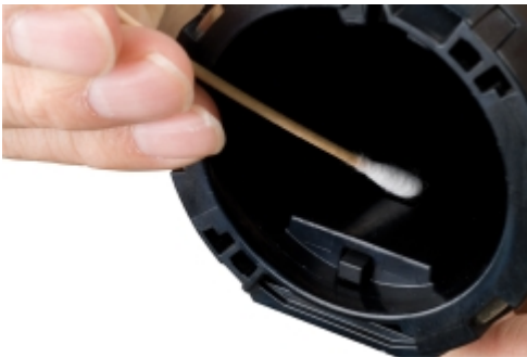
Figure 22 Calibration cap diode cleaning
