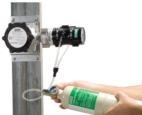
Figure 11 Bump Check setup with environmental guard
