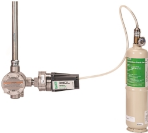
Figure 10 HART Calibration Cover/Bump Cap
