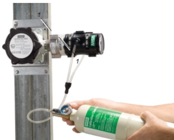
Figure 16 HART calibration set-up
